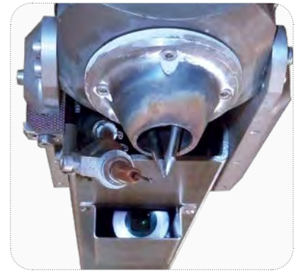
TIG er lance with integrated camera
