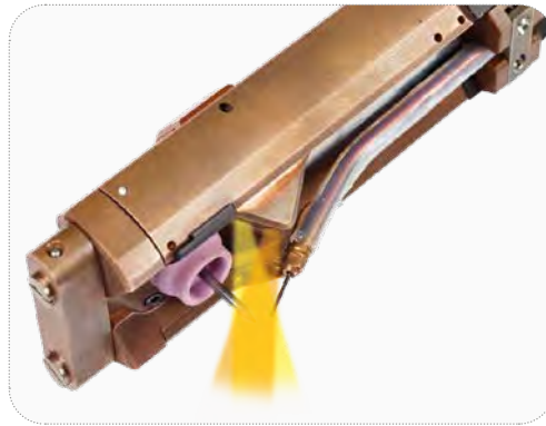
TIG lance with integrated camera and light
